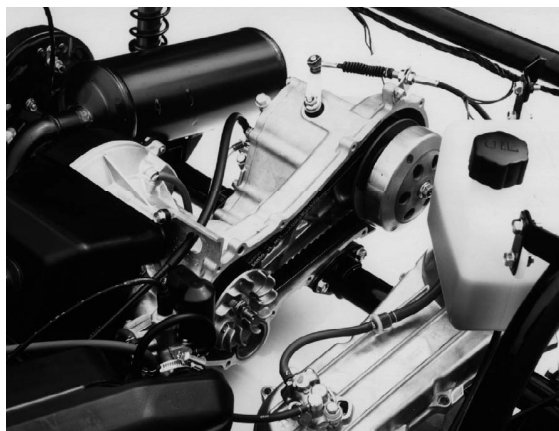
◀ for motor bike Variable speed belt
