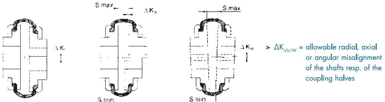
> Radial misalignment    > Axial misalignment    > Angular misalignment
