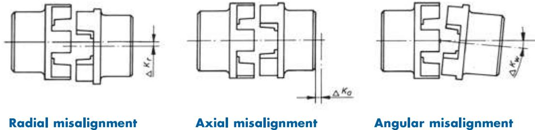
► Reduction of the allowable values of misalignment when the combination of misalignments occur or at other rotational speeds:
