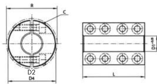
> Material, design: steel 1.0718, black-oxided; stainless steel 1.4305, blank
