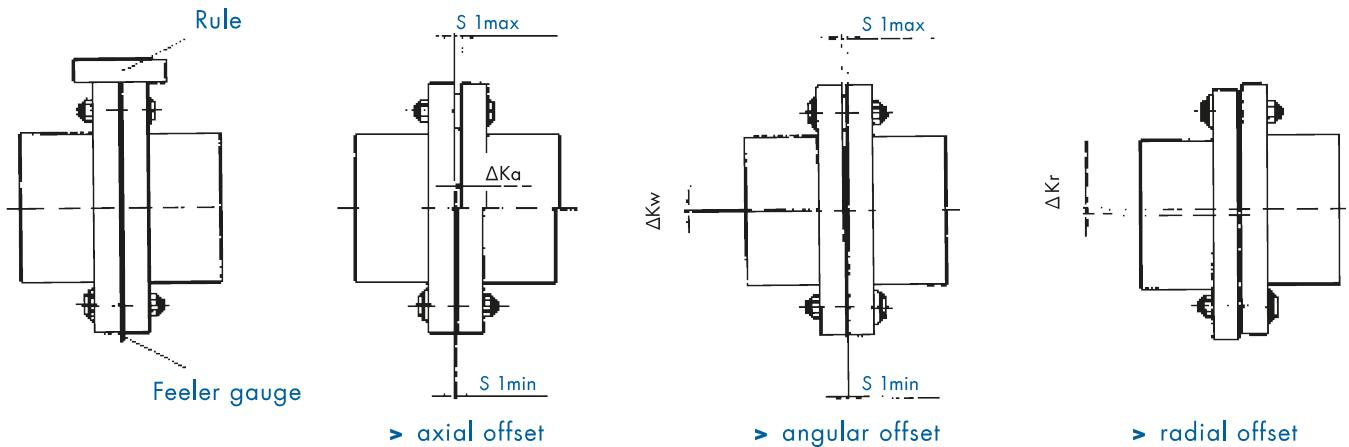
Offset of coupling parts in relation to one another may arise from an imprecise alignment during assembly, but also from operation of the machine (thermal expansion, shaft sag, excessively soft machine frame etc.).
